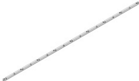
M01 LOUVER MOUNT - A4M02593 (x1) 1"x1 15/16"x110 3/4" (25x49x2813)
