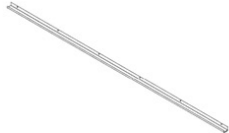
G01 GUTTER - A4M01993 (x2) 1 9/16"x1 15/16"x108 7/8" (40x50x2765)
