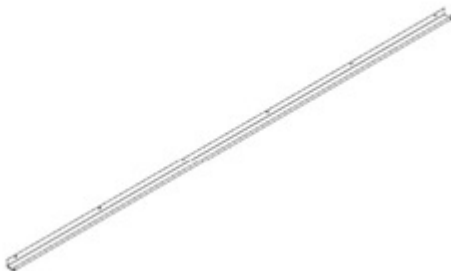
G02 GUTTER - A4M02583 (x4) 1 9/16"x1 15/16"x111" (40x50x2819)
